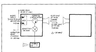
fig. 1. The Gunnplexer consists of a Gunn-diode oscillator, which serves as both the transmitter and receiver local oscillator, and a Schottky diode and ferrite circulator which are used as the receiver mixer.
